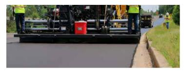
**Stretch® 16 Screed with zone Electric heating** offers absolutely uniform heat distribution for a quality mat. The flexible paving width of 8- to 16-feet makes the CR 821 W ideal for a variety of applications. Stretch® 16 Screed has wear-resistant, durable steel plates for long lifespan and reduced maintenance.
